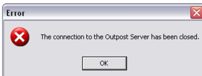
Fig 38 – Automatic closure of an inactive connection
